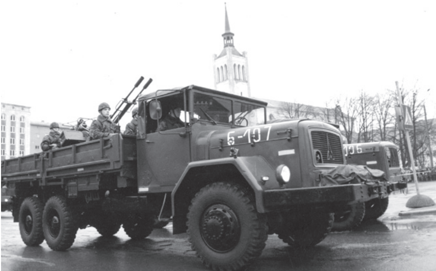
Estonian air defence troops with a Soviet towed 23 mm anti-aircraft twin-barrelled automatic cannon Sergey ZU-23-2 in a German Magirus truck trailer. Estonian bought these anti-aircraft autocannons from Israeli company IMI-TAAS (1997). Rauno Volmar/Estonian Defence Forces
